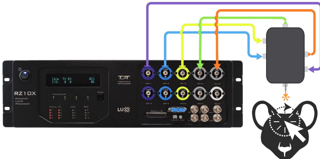
Connection diagram for a 3-color fiber photometry setup.
